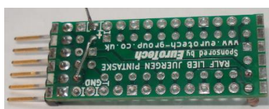
47k resistor, body to the inside as shown
