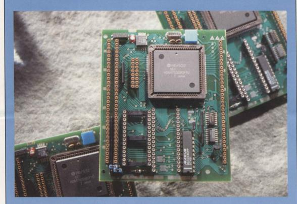
As a **Data Collection Module** with removable Card Memory option, you've little to add to its 10-bit 8-channel analog to digital converter, real time clock and memory of up to a gigabyte.
